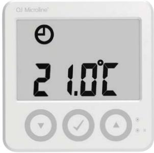
WLDT is a room sensor with display. It displays and controls room temperature with the possibility of adjusting the standard set point in the system by  $\pm 4^{\circ}\text{C}$ . It also features mode selection, where Auto, Day, Night and OFF (frost protected) are available, and allows connection of a floor sensor for minimum or maximum floor temperature limitation.
